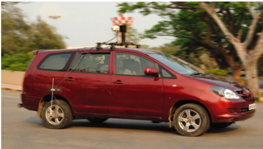
Figure 3.2: iRAP Navigation Survey Vehicle
