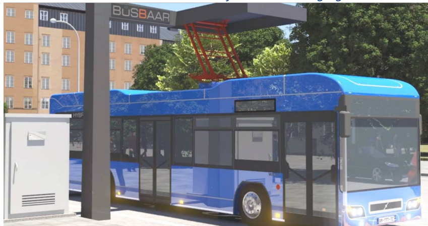
Picture 32 - BusBaar - bus station fast charging.
